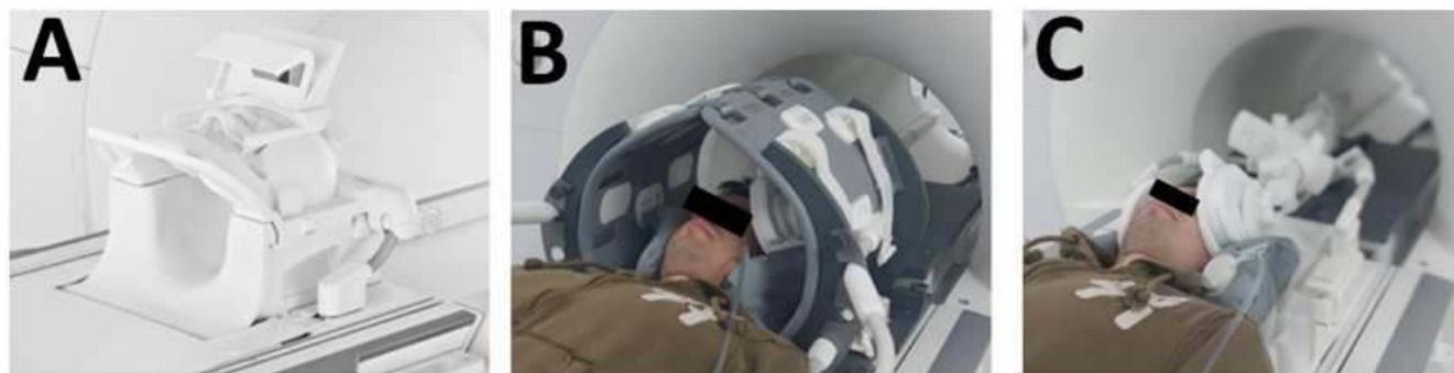
Three different coil setups used: A) standard 64ch head-neck coil, B) two 18ch body array coils wrapped around the head using a home-built coil holder, C) commercially available MRI-TMS coil consisting of two 7ch coils combined with a MRI compatible TMS brain stimulation coil
